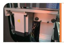
AC Servo Motor driven trolly movement.
